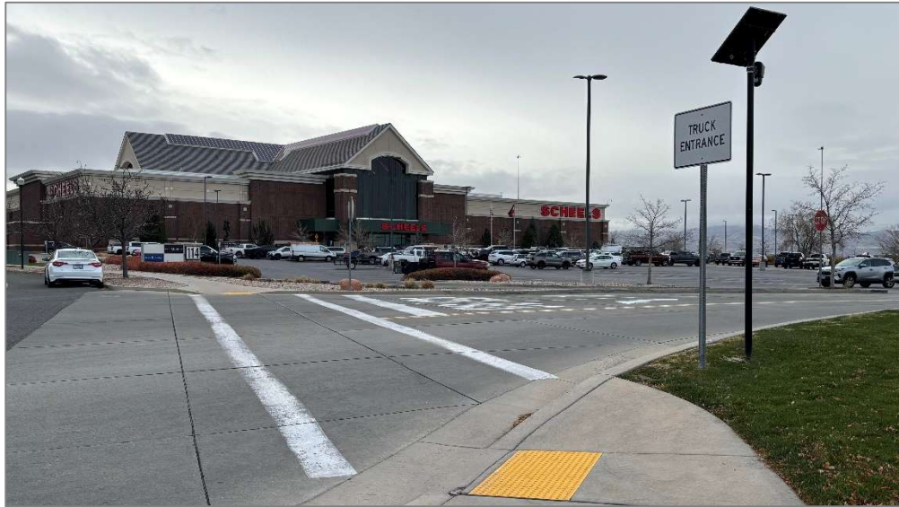
Figure 13: Truck entrance sign at Scheel's access is not MUTCD-compliant
