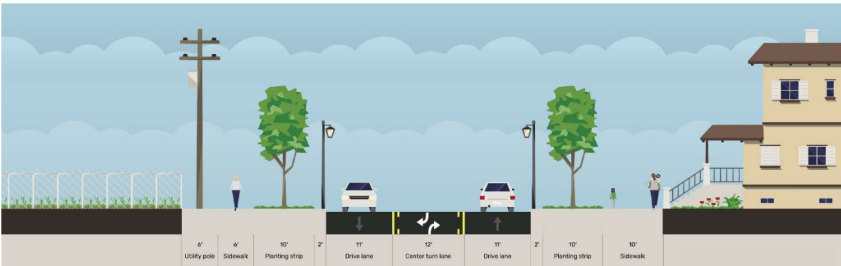
Alternative Cross Section – Planting Strips and Lighting
